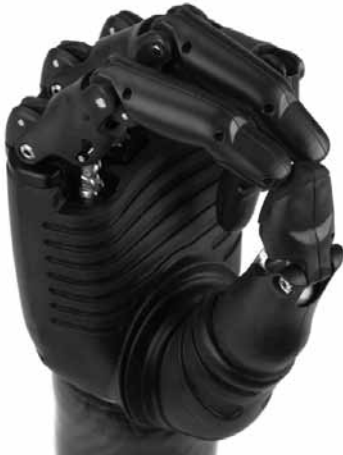
Improved Tripod Grip - improved positioning facilitates secure hold on thin & small objects
