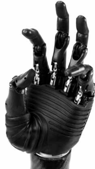
Mouse Grip - allows index finger to left click on computer mouse while little finger and thumb secure grip
