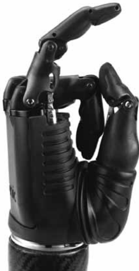
Trigger Grip - allows index finger to flex for trigger actuation while other fingers grasp handle. Not for use with firearms.
