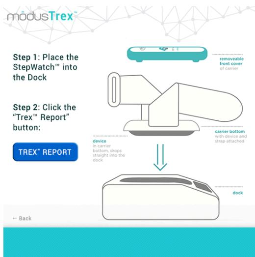
Do not remove the monitor from the dock while it is communicating (while the red light on the dock is on).
